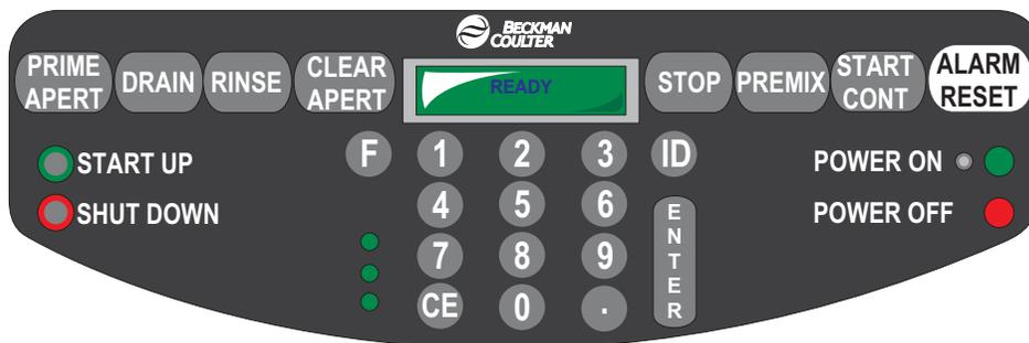
The Analyzer contains a keypad and a small Liquid Crystal Display (LCD). Use the keypad to initiate Diluter functions or provide numeric values.
