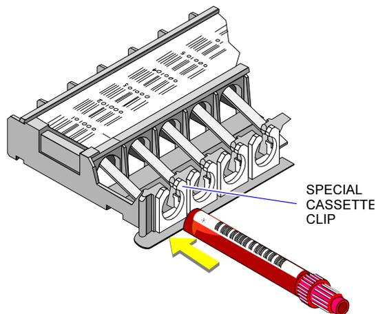
Make sure the bar-code label faces up when you place a tube into the cassette so that it can be scanned correctly.
