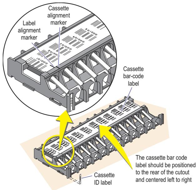
The cassette is the carrier for the sample tubes (patient, control, or special test) used in Automatic aspiration mode where automatic loading, mixing, and sampling occurs.
