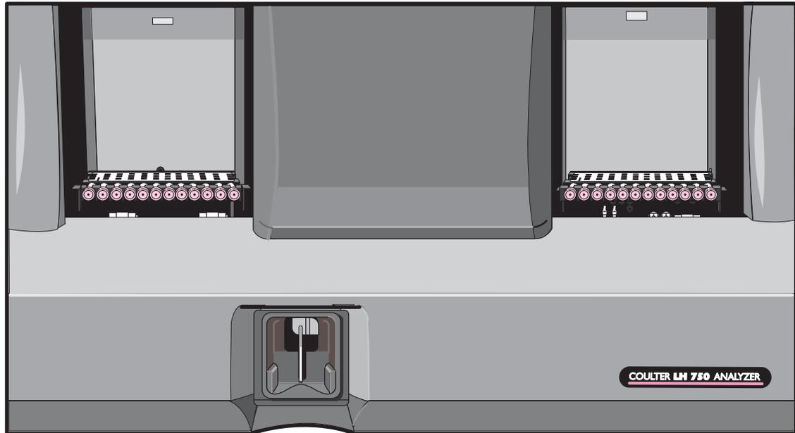
This is the fluidics portion of the LH 700 Series System. The Diluter is the subsystem that aspirates the sample, dilutes it and mixes it. Move the cursor over the illustration to see links to additional information.
