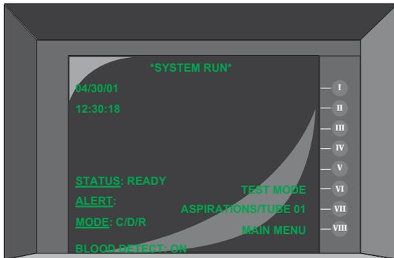
The Analyzer has a set of CRT buttons and a screen. The screen displays messages and menu items. Press the buttons to the right of the screen to perform LH 700 Series System functions.
