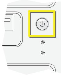
Before turning the Workstation off, you should try to shut down the Workstation to avoid loss of any data. If you cannot shut down the Workstation, turn the Workstation off, wait 30 seconds and restart the Workstation.
