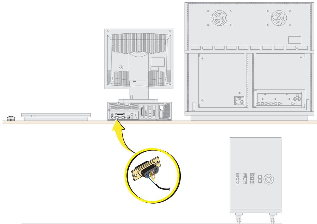
**Note:** The DB 9-pin connector on the computer base, designated as COM 1, is located beside the video display connector.
