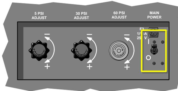
Master circuit breaker enables/disables input power reaching internal electrical components of the Power Supply.
