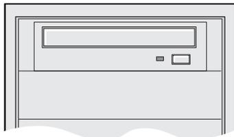
Your Workstation uses a Compact Disk Read-Only Memory disk drive to read data from a CD ROM disk, such as the Audio Visual Help CD-ROM. This CD-ROM holds text, graphics and hi-fi stereo sound.
